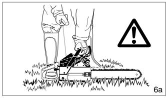
Place the chain saw on firm ground or other solid surface in an open area. Maintain a good balance and secure footing. Place your right foot through the rear handle opening and firmly grasp the front handle with your left hand (fig. 6a).
